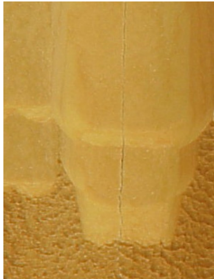
Figure 7. Transverse-cracking failure mode.*
