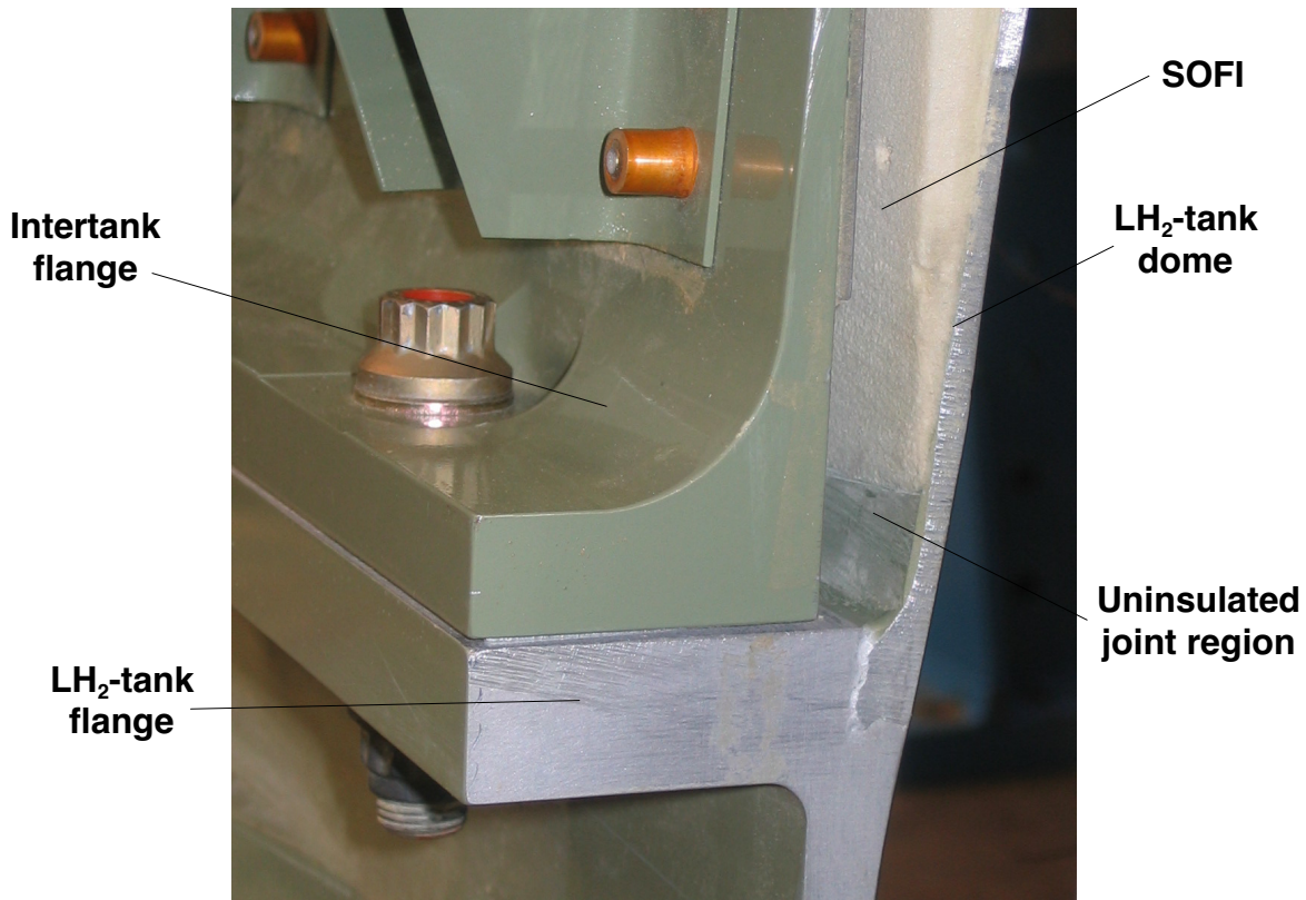
Figure 2. Cutaway of the Y-shaped joint between the liquid hydrogen tank and the intertank structure.
